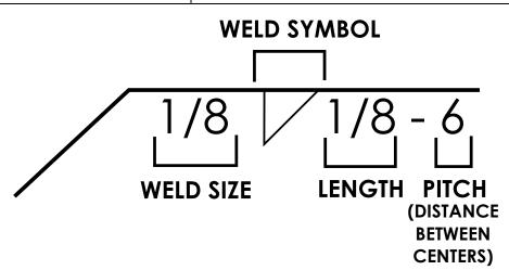
This symbol tells us to make a 1/8" high Fillet Weld, 1/8" long (a "tack"), and to do so along the seam every 6" (the pitch).
