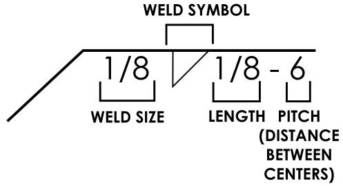
This symbol tells us to make a 1/8" high Fillet Weld, 1/8" long (a "tack"), and to do so along the seam every 6" (the pitch).
