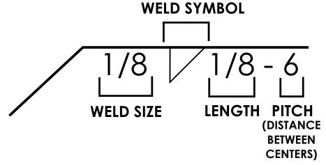
This symbol tells us to make a 1/8" high Fillet Weld, 1/8" long (a "tack"), and to do so along the seam every 6" (the pitch).
